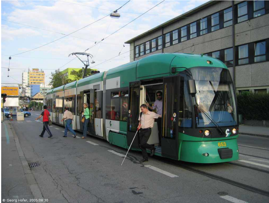
Figure 2- Use of a low-floor tram with no platform, Graz, Austria. Georg Hoffer photo.
