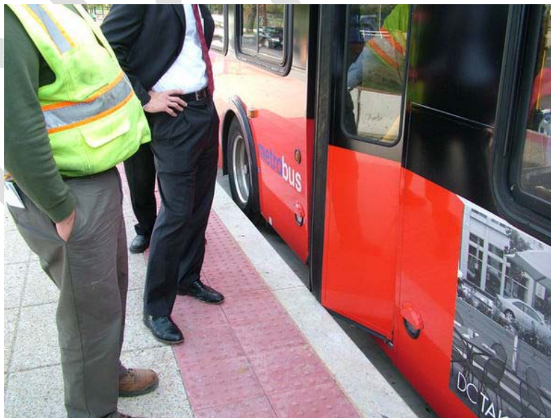
Figure 5- Rear doors on bus blocked by 355mm (14 inch) streetcar platform
